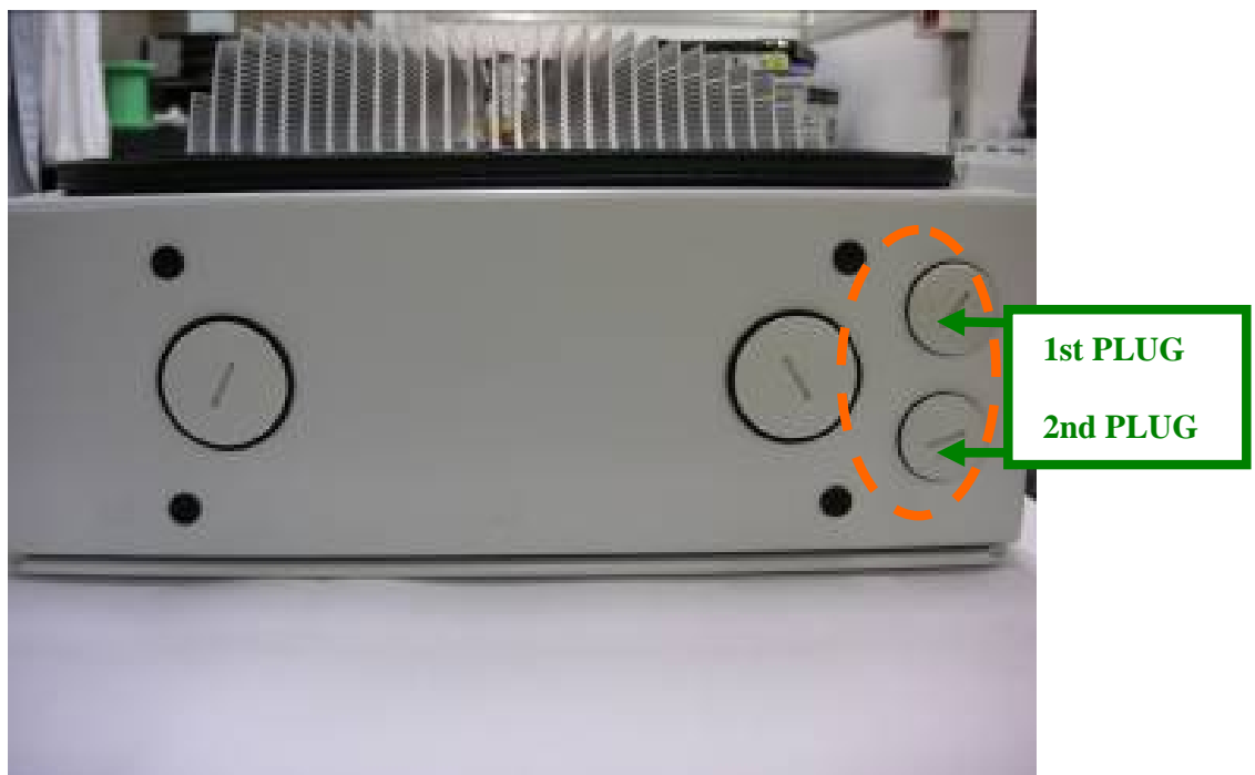
Fig.23 - Holes for cables necessary for RS-485 port connection or wiring for RJ12 connectors connection.
