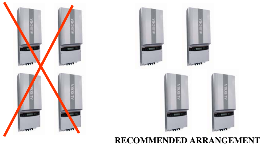
Fig.7 - Recommended installation of AURORA inverters
